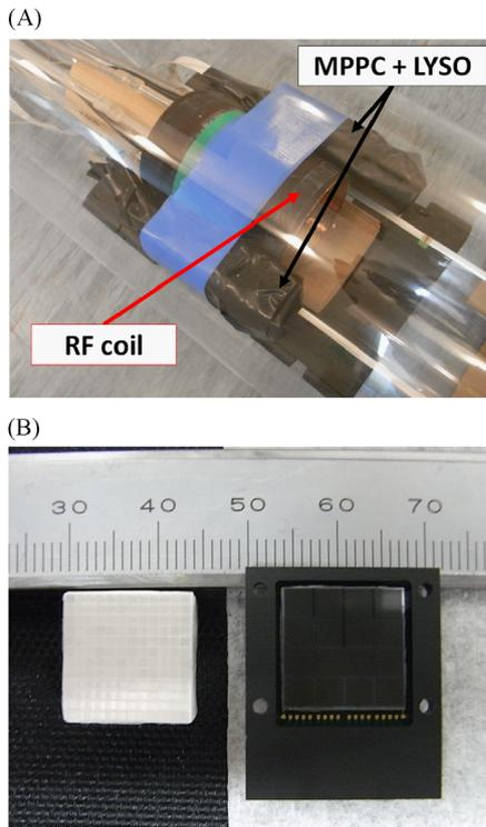
**Fig. 1.** Left: A pair of MPPC modules was positioned around the RF coil. Right: LYSO scintillator array and MPPC array. This scintillator array is fabricated into 12 × 12 matrices of 1 × 1 mm pixels. The MPPC array is the model number of S11827-3344MG (Hamamatsu Photonics K.K.).
