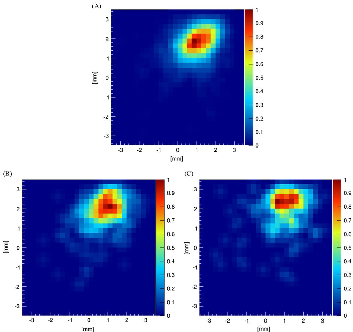
**Fig. 5.** The image of a point  $^{22}\text{Na}$  source. (A) The MPPC module is outside MRI. (B) The MPPC module is inside MRI under FSE. (C) The MPPC module is inside MRI under GE. (A) outside MRI, (B) under FSE and (C) under GE.
