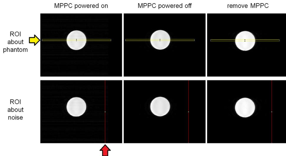
**Fig. 6.** The MR images (Cooperation of BioView Inc. (Japan)). These are the images when the MPPC module powered on is inside the MRI (left), when powered off inside the MRI (center), and when removed from the MRI (right). The top and bottom rows show the region of interaction between phantom and noise, respectively. (For interpretation of the references to color in this figure legend, the reader is referred to the web version of this paper.)
