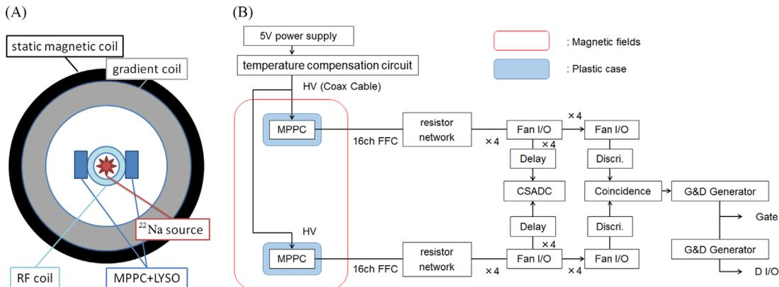
**Fig. 2.** Left: The experimental setup used for the imaging tests of PET. Right: The block diagram. We apply a voltage to the MPPC by passing through a 6-m coaxial cable. The signals from the MPPC pass through a 5-m flexible flat cable.
